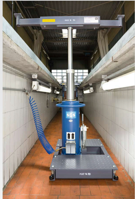
TKS 14/1200 FV-Q with axle cross beam ATB V-16 Axle cross beam not supplied
